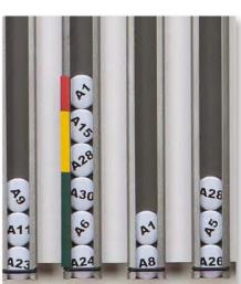
Detail FiFo row equipped with coins and magnetic strips in traffic light colours
